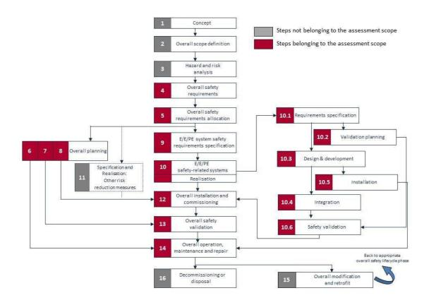
The ball valves are generic products that could be used in a complete safety loop. Chapters 1, 2, 3, 11, 14, 15 and 16 are not included in the area of assessment and fall under the responsibility of the final client.
